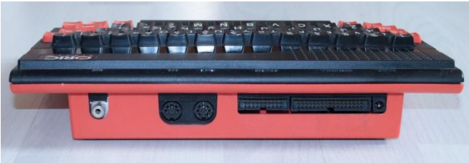
The interfaces: HF, Tape & RGB, Centronics and system bus
